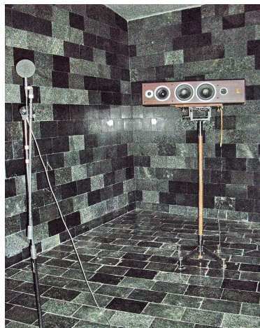
Measurements in reverberation room
