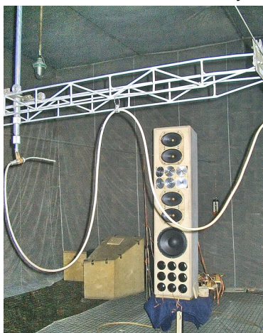
Measurements in anechoic chamber
